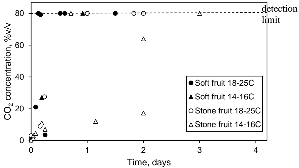
Figure 2.2.3. Carbon dioxide concentration in the headspace of sealed bins containing fruit waste
